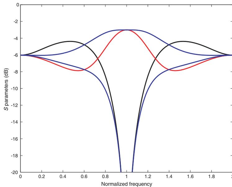
Figure 2: Frequency response of the 3 dB directional coupler.
